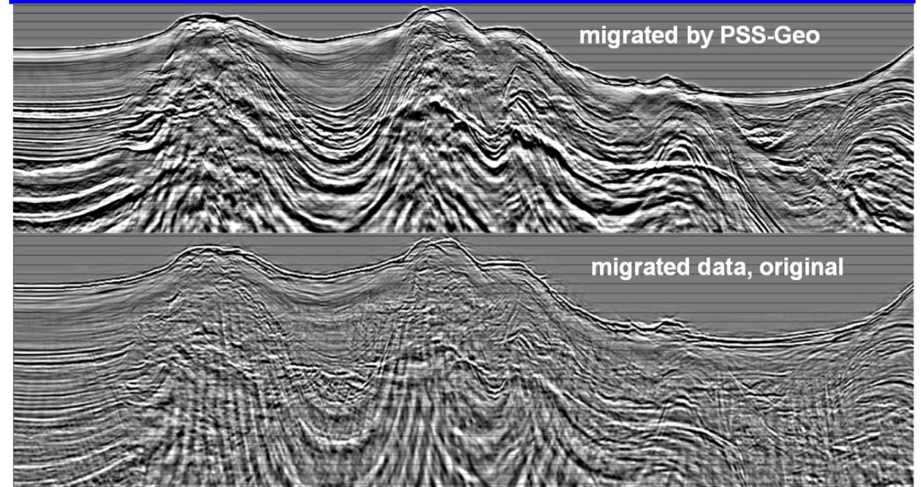
Top picture is seismic data processed by PSS-Geo AS. Migration algorithm is old known Kirchhoff Anisotropic Wavefront Propagation Depth migration. Velocity model is corrected velocity model built by using logs data and anisotropic VTI/TTI gridded tomographic solution through iterations approach. Bottom picture is the same seismic data migrated by modern algorithm with simplified velocity model.
