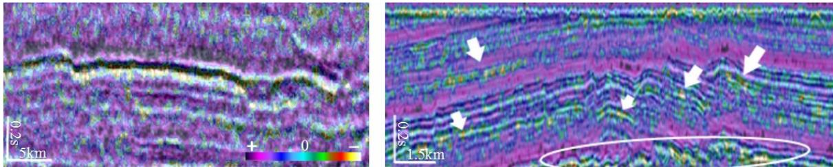
**Figure 5** Q-factor sections: Stetind gas field, Norwegian Sea (left), Korpffjell, gas, Barents Sea (right).
