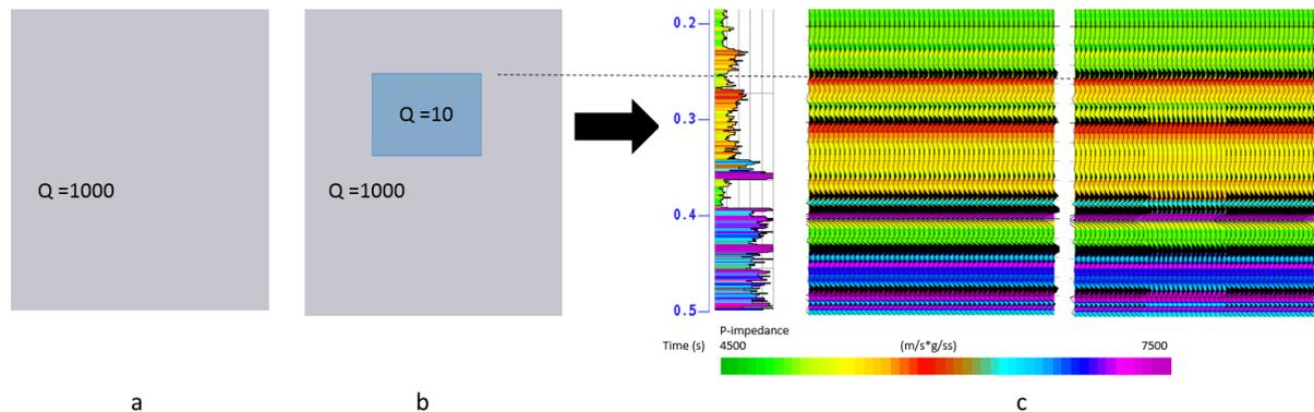
**Figure 1** Media models and their synthetic seismograms. a - Plane model, b - Model with absorption block inserted ( $Q=10$ ), c - P-impedance log used to generate synthetic traces; synthetic of Plane model and of Model with absorption area inserted. Wavelet parameters used to generate synthetic trace: Bandpass wavelet 5-10-40-125 Hz, 2ms sample rate and 100ms length.
