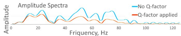
**Figure 2** Amplitude Spectra for Plane Model and Model with absorption block inserted. Model with Q-factor (red color) has less amplitude values - damping amplitudes. The biggest damping occurs for higher frequencies.
